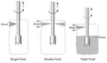
Fig. No. 17 shows types of drilling pipes
