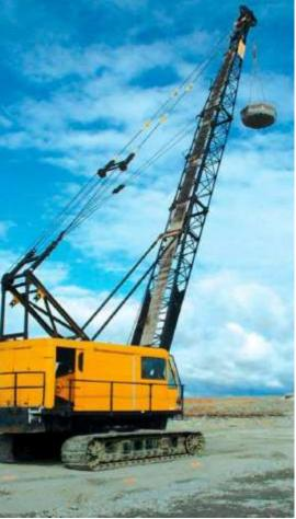
(Fig. No.12) Demonstrates the equipment used in the Dynamic consolidation method
