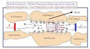
Figure No. 14: shows the effect of the electric field on the movement of groundwater in the clay layer
