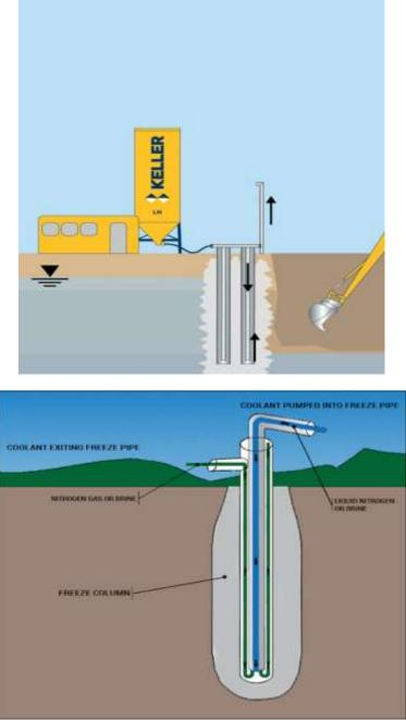
Figure No. (19) soil improvement by freezing
