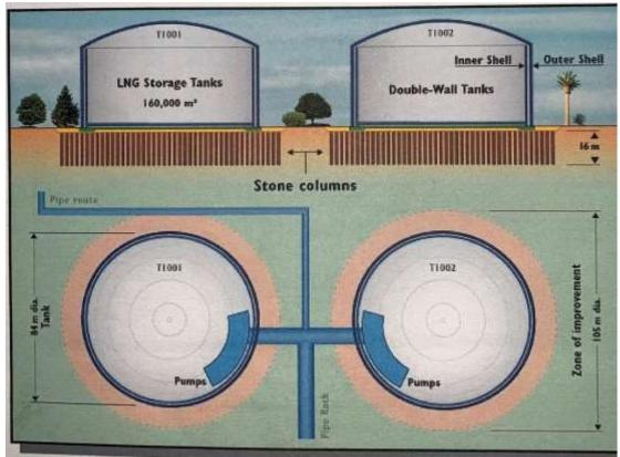
Figure No. (7) reservoirs whose foundations were executed by the stone column method
