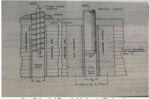
Figure (9) shows the drilling methods for the vertical filters' operation
