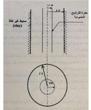
Fig. No.11 Diagram showing the dimensions of the filter column and the circular area it serves
