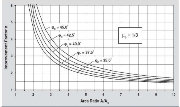
Figure No. (5) a graph showing the relationship between the degree of soil improvement and the column diameter for different types of soil
